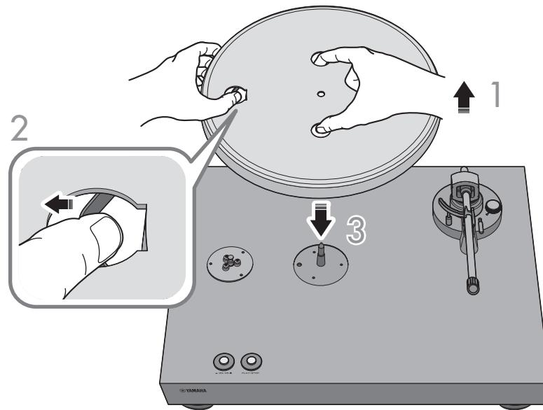
**4 将转盘底座的圆孔对齐滑轮。**
